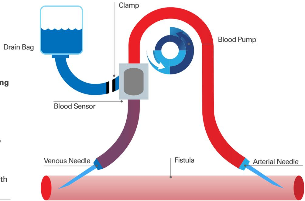
**Figure 4. Variation of Blood Priming Without a Blood Sensor**
